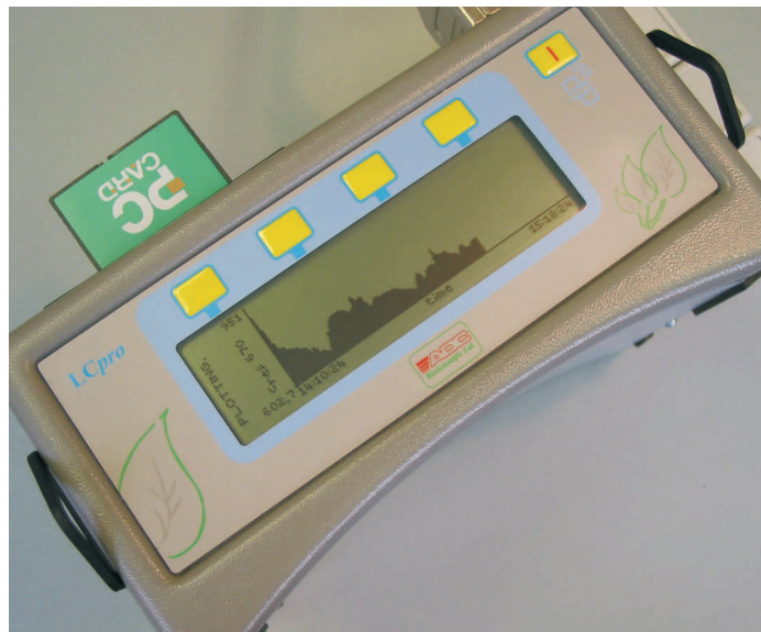
Five Buttons scroll through menu driven software.
