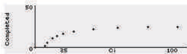
Typical A/Ci curve that can be produced by the LCpro +
