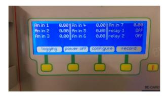
Gas readings, flow indication, power supply status and date and time are all displayed on the main menu screen. Configuration and control is by simple to use, menu driven software
