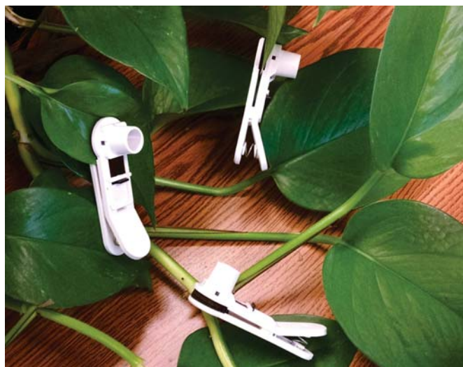
Dark adaption clips - The F V /F M meter comes with 10 clips. Clips are available individually or in packages of fifty.
