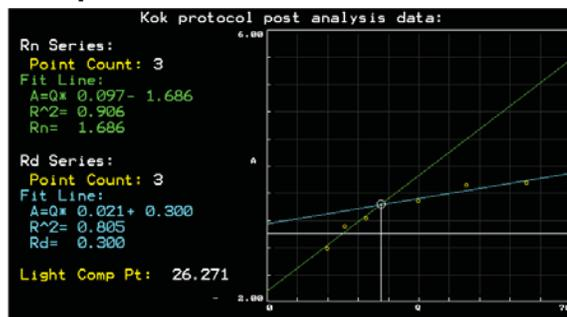
The Kok protocol can be used for  $R_d$  determination. It is primarily used in  $C_4$  plants, but it has also been used for  $C_3$  plants. The Laisk protocol is considered more authoritative for  $C_3$  plants. Least squares linear regression analysis algorithms are included to provide the graphing and results shown on the screen.
