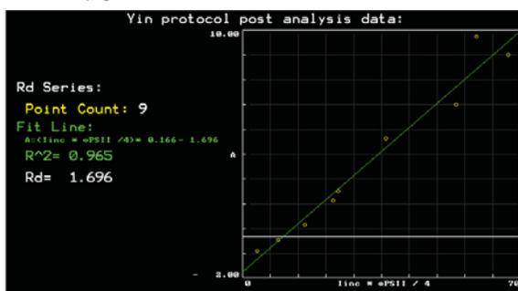
The Yin Protocol is a more recent approach that uses the combined measurement of gas exchange and chlorophyll fluorescence to determine  $R_d$ . It offers the advantage that higher light levels and  $CO_2$  levels can be used. Under these circumstances, errors are perceived to be smaller in relation to the values measured.
