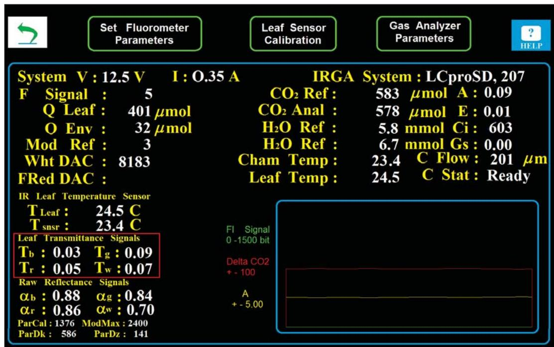
Here, T<sub>b</sub> is the portion of leaf transmittance in the blue spectrum, T<sub>g</sub> is the portion of leaf transmittance in the green spectrum, and T<sub>r</sub> is the portion of leaf transmittance in the red spectrum. α<sub>b</sub>, α<sub>g</sub>, α<sub>r</sub>, values represent leaf absorptance using reflectance only in their respective μm color ranges. Absorptance displayed in all protocols use both reflectance and transmittance values for calculation.
