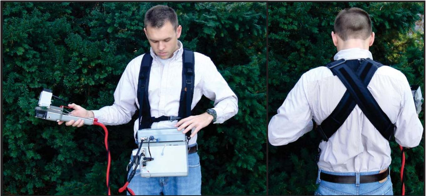
The all day instrument harness is available as an accessory for those researchers that plan to take a number of individual measurements over longer periods of time. It is designed to distribute the weight of the instrument evenly across the back and over both shoulders. The back cross design, also found in high quality backpacks, allows comfortable working conditions for hours. To help prevent headaches, there is no strap across the back of the neck.
