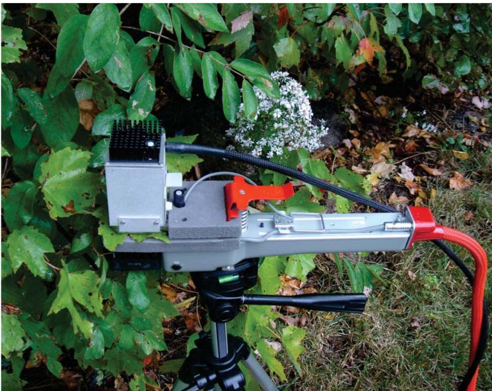
There are dual PAR sensors; one inside the fluorometer chamber, and one for ambient measurement. This allows for the option of using the instrument to measure ambient light levels, and duplicating the level in the chamber. One can significantly reduce the time to reach ambient steady state photosynthesis.
