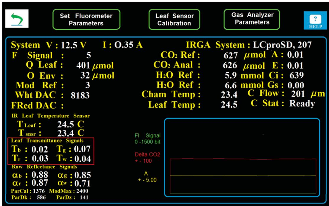
The screen above shows leaf transmittance values in the blue, green and red parts of the spectrum on an indoor leaf, at near saturation light levels of 400 μmolls, after 4 minutes. The lower screen shows transmittance values after chloroplast migration, or after 35 minutes. Notice the change. Leaf absorptance changes with light intensity! (Cazzaniga 2013) & (Dall'Osto 2014)
