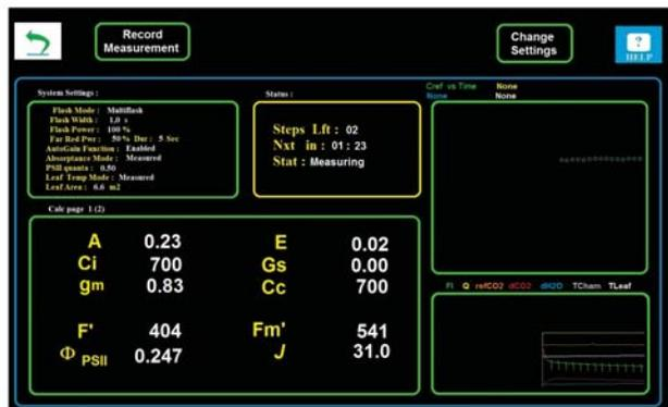
Measuring screen with calculated measuring parameters including  $g_m$  and  $C_c$ .
