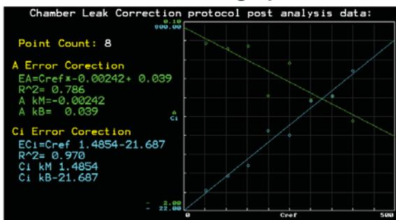
When measuring  $g_m$ ,  $C_c$ ,  $R_d$  and  $\Gamma^*$ , system chamber leakage & dark respiration diffusion from under system gaskets become important. The Flexas chamber leakage protocol lets the researcher test instrument chamber leakage, for the species being tested, and *automatically apply the results* to other tests and protocols that follow.
