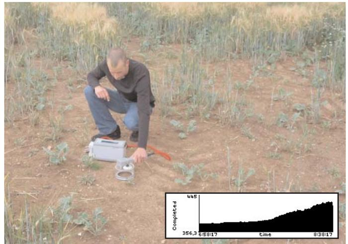
Full functionality, flow control and data logging are all contained within the compact console. Experimental programming and operation is achieved with just five keys to drive a series of simple menus. All soil respiration data and calculations are clearly presented on a large high definition liquid crystal, graphic display.
